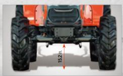
High Ground Clearance The maximum ground clearance of 15.2 in. makes usage on rocky or uneven terrain simpler.
