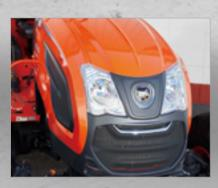
Center Marker The center marker on the hood assists with maintaining straight rows.
